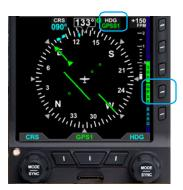
Figure 6-9 Operating in GPSS Mode
