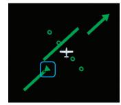
Figure 4-38b 360° and ARC FROM Indication (without Reduced Length Course Pointer)
