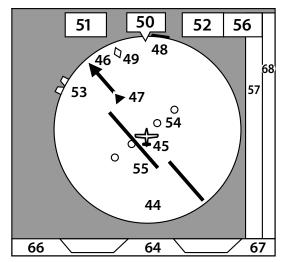
Figure 2-25 Navigation Display Components
