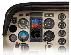
Figure 1-2 Single Display Evolution E5 Dual EFI
