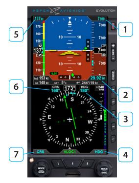
Figure 2-3 Left and Right Knobs and Corresponding Fields
