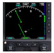
Figure 4-33 ARC Compass Mode
