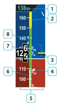
Figure 4-11 Airspeed Indicator
