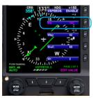
Figure 5-13 Va Vspeed Set With New Value
