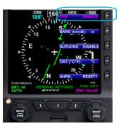
Figure 4-16 **Editing Airspeed Tape Display**
