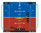
Figure 4-28 Airspeed and Altitude Tape Disabled
