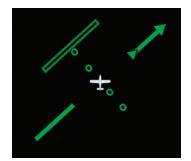
Figure 4-41 Deviation Exceeded, 360° and ARC Compass Modes
