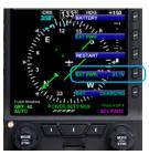
Figure 6-4 External Power Voltage Status
