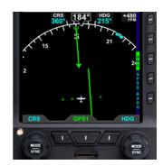
Figure 4-35 ARC Compass Mode
