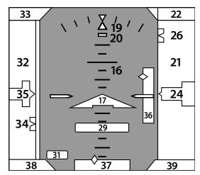
Figure 2-20 Attitude Display Components
