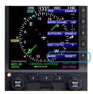
Figure 6-7 AHRS Reset Menu Key
