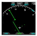
Figure 4-37 Reduced Length Course Pointer, ARC Compass Mode
