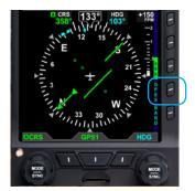
Figure 4-65 GPSS Disabled and Autopilot in HDG Mode
