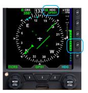
Figure 4-64 GPSS Enabled with Autopilot in HDG Mode
