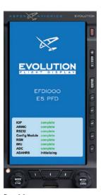
Figure 3-2 Evolution E5 Dual EFI Initializing
