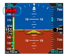
Figure 6-3 Battery Charge Remaining
