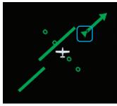
Figure 4-38a 360° and ARC TO Indication (without Reduced Length Course Pointer)
