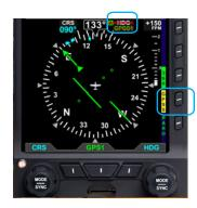
Figure 6-10 GPSS in Wings Level Mode
