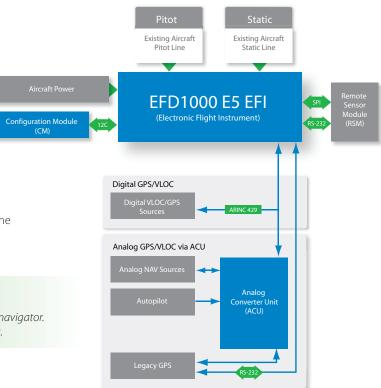
Figure 1-2 Evolution E5 Dual EFI System Architecture
