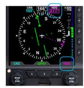
Figure 3-8 Selected Heading Field Enabled
