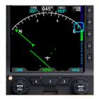
Figure 4-52 Selected Heading Bug Outside of the ARC Compass Scale Range
