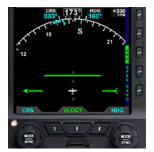
Figure 2-31 ARC compass mode
