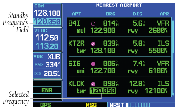
Figure 8-7 Frequency Moved to Standby Field
