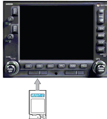
Figure A-2 Data Card Insertion/Removal Detail
