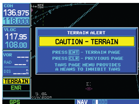
Figure 13-3 Caution Alert Pop-up
