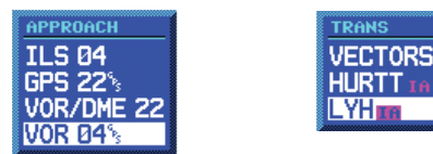
Figure 6-11 Approach and Transitions Windows
