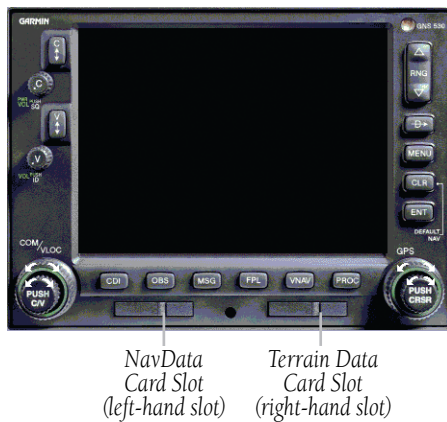
Figure A-1 Data Card Slot Locations
