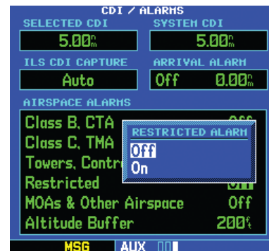
Figure 10-31 Restricted Alarm Window
