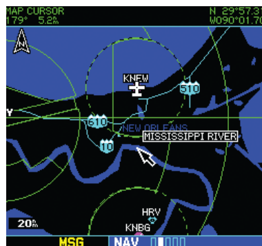
Figure 7-41 Activate Panning Function
