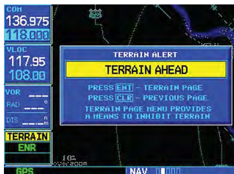
Figure 12-4 TERRAIN Caution Pop-up (Flashing)
